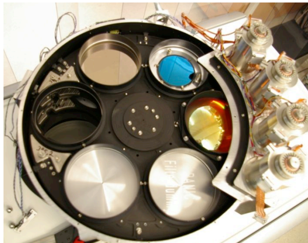
Figure 5: Image of filter wheel 1 equipped for lab testing. It is populated with filters Ks (top left), H (top right, smaller diameter, from the instrument Omega2000), the PIL (right), and two dummies. The open position is on the left.
